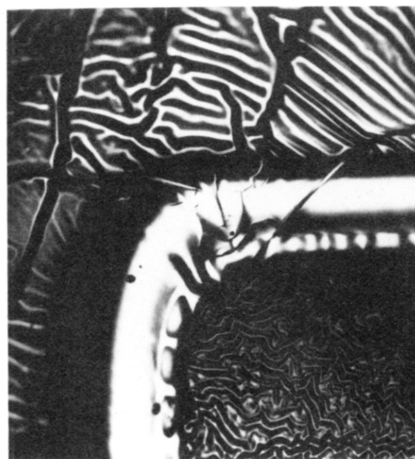
Figure 4. Optical micrograph of SIMS crater.
